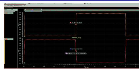
Inverter Delay here measured between 50% of input to 50% of output.
