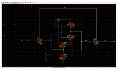
6T-SRAM consists of 2 Inverters and 2 Access transistors.
