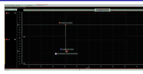
The delay is calculated as time difference between 50% of input to 50% of output. The delay is 10.84ns.
