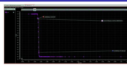
The fall time is calculated as time difference between 90% of maximum voltage and 10% of maximum voltage. The fall time is 351.9ps.
